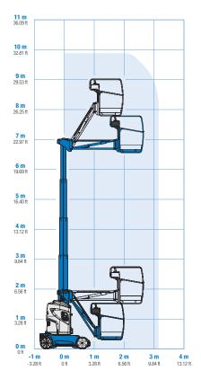
\* The metric equivalent of working height adds 2 m to platform height. U.S. adds 6 ft to platform height.
