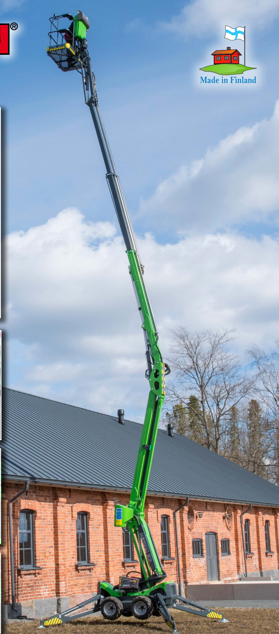
New tailor made trailer for L190, axle capacity 3500 kg
